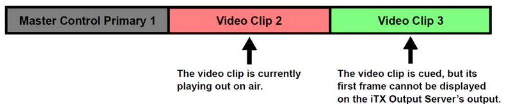
Fig. 2-7: CTFF does not occur if the current playout event is also a video clip from the iTX Output Server
