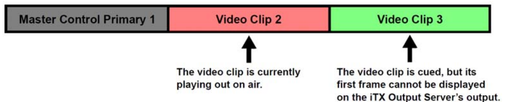
Fig. 2-7: CTFF does not occur if the current payout event is also a video clip from the iTX Output Server
