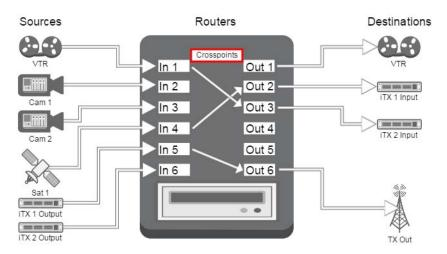
Fig. 5-1: How channel sources and destinations connect to a matrix router.
