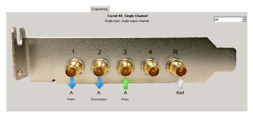
Depending on the selected playout type, Corvid 44 video/audio I/O cards uses the following inputs and outputs:
