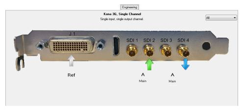
Kona 3G video/audio I/O cards only support the single channel playout type and have the following inputs and outputs:
