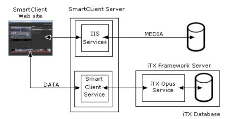
In a typical system, the SmartClient Service will run on its own Windows 2008 Server machine together with the IIS components and other prerequisites required for the installation. The SmartClient Service will communicate with the Framework Server's Opus Service by either of the existing 'Discovery' or 'Locator' methods.
