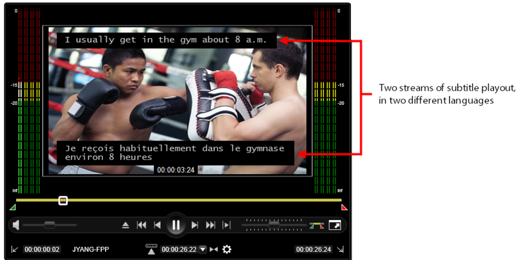
Fig. 8-2: The Preview as Channel media player, showing the playout of two subtitle streams.
