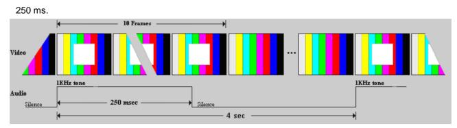
Figure 5.51 Lip Sync test signal appearance and timing
