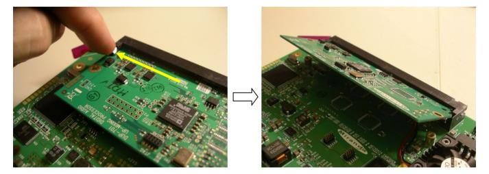
4. Pull the module out of the socket
