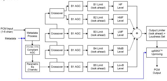
**Figure 6.11** General signal flow of the AeroMAX<sup>TM</sup> processing core
