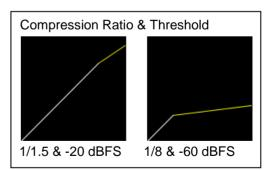
Use the *Ratio* pulldown to set the compression ratio (i.e. slope of the transfer curve). The compression ratio specifies how much the output level changes with respect to the input level:
