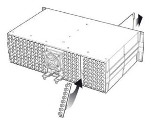
Figure 2.1 Densité-3 frame – rear panel installation
