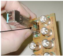
3. Slide the module straight into the socket, and push gently until it clicks into position.
