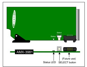
Figure 1.2 Front card-edge layout
