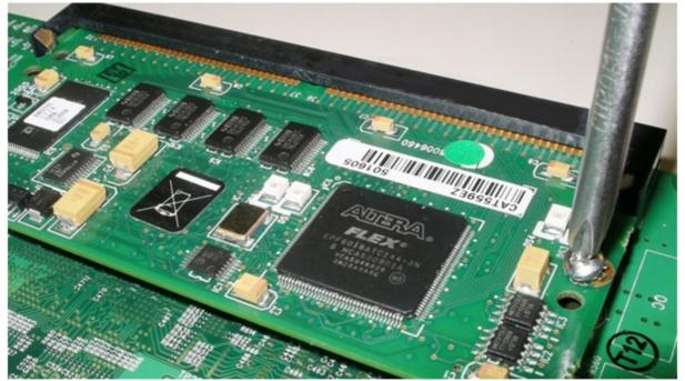
3. Push outward on the two metal clips that hold the module in the horizontal position, one located at each corner of the socket. The module will release and tilt upward
