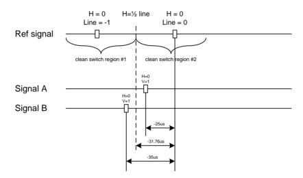
*Example 2:* We have two SD (525) sources, one that indicates an offset of  $50\mu s$  with respect to the reference (A) and the other an offset of  $40\mu s$  (B). We know that a clean switch region limit is present at +  $\frac{1}{2}$  line and another one at  $\frac{1}{2}$  line plus one line. These correspond to  $31.76\mu s$  and  $95.28\mu s$ . We can now determine that this switch will be clean, because the two sources are inside the same clean switch region.
