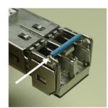
2. Position the SFP module so that the recessed slot is lined up with the tab side of the socket.
