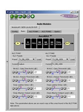
• **ITU LOUD**ness **LMT** - Utilizes a specially tuned Input AGC plus Multiband Limiters and the Final Limiter to slowly adjust the average program loudness to a given value and the multiband and final limiters will act until the AGC catches up. This preset is appropriate for ingest or live applications but because the Multiband AGC is bypassed it has less ability to manage spectral balance which is important for transmission.
