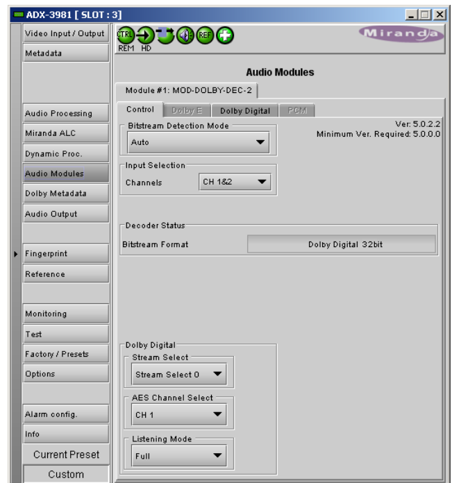
Figure 6.1 Audio Modules - Dolby Decoder - Control
