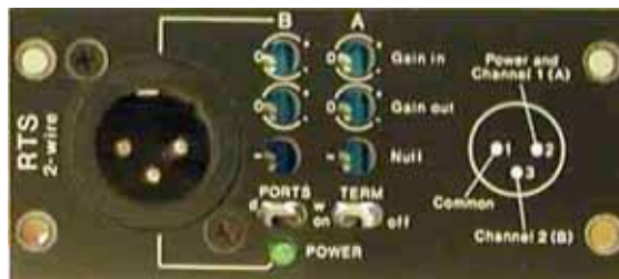
Figure 29: Intercom Module: RTS Telex
