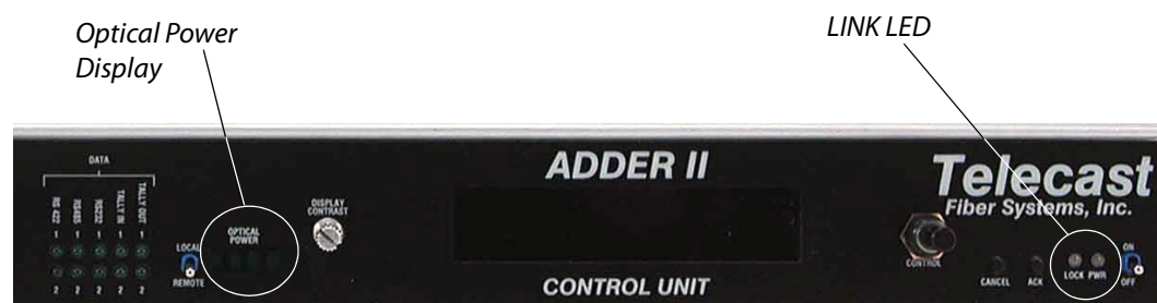
Fig. 2-3: Optical Power Display and LINK LED Location, Front panel
