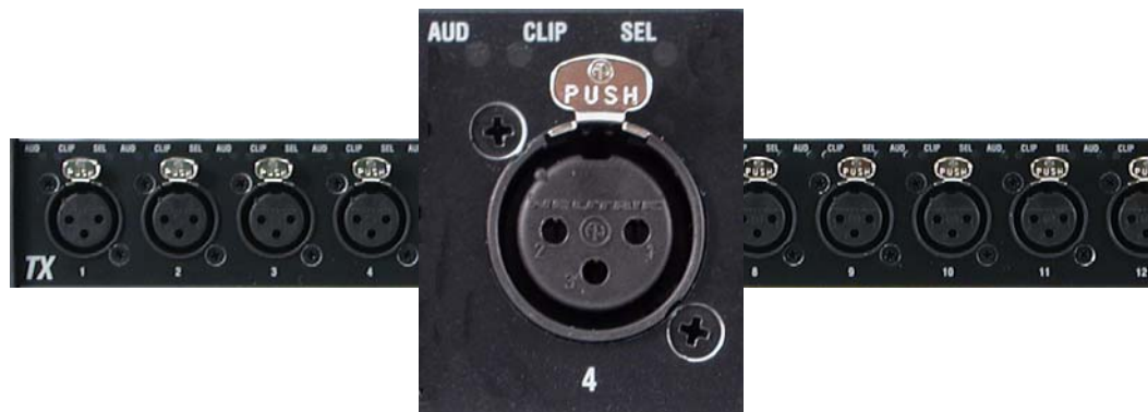
Fig. 2-13: Analog TX Module and Analog TX LED indications
