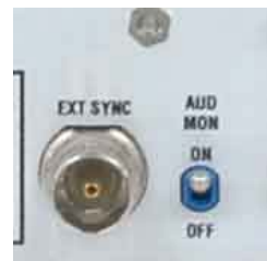
Fig. 2-10: AUD MON On/Off Switch
