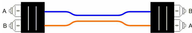
A-to-B duplex optical fiber patch cord Continuous Fiber Position (A-B, B-A) ANSI/TIA-568-C
