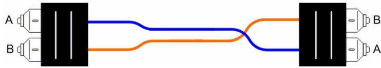
A-to-A duplex optical fiber patch cord Reverse Fiber Position (A-A, B-B)
