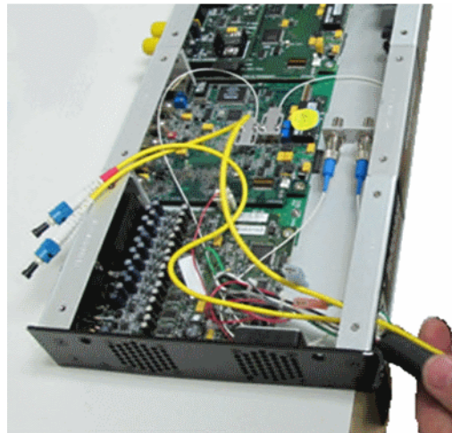
Fig. 2-8: Feeding the wire into the chassis
