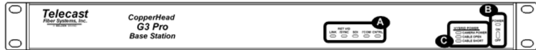
Fig. 3-8: Base Station Front Panel - single unit, 120/220 VAC power w/internal hybrid power supply
