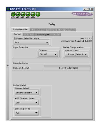
The *Input Selection* determines the Dolby decoder input channel pair. Channels 1 to 8 represent the AES1 to AES4 digital inputs. When a video card is present, eight extracted audio channels are available as channel 9 to channel 16. See *Audio Processing/Config tab* for the input selection from the video card.
