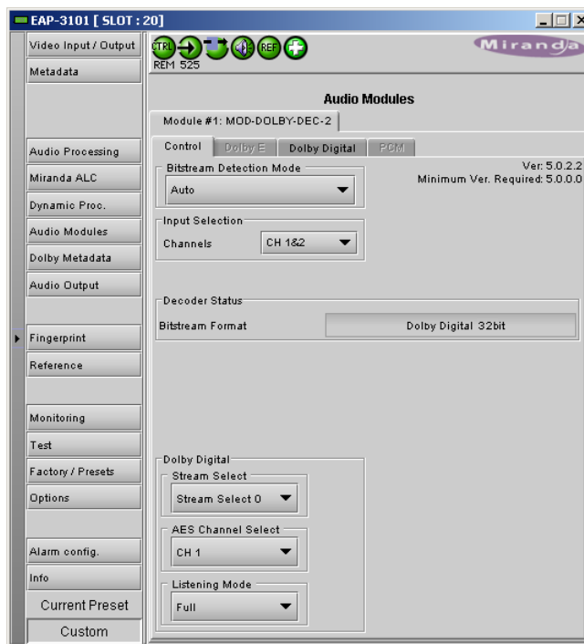
Figure 6.1 Audio Modules - Dolby Decoder - Control
