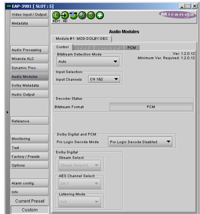
Figure 6-1 Audio Modules - Dolby Decoder - Control
