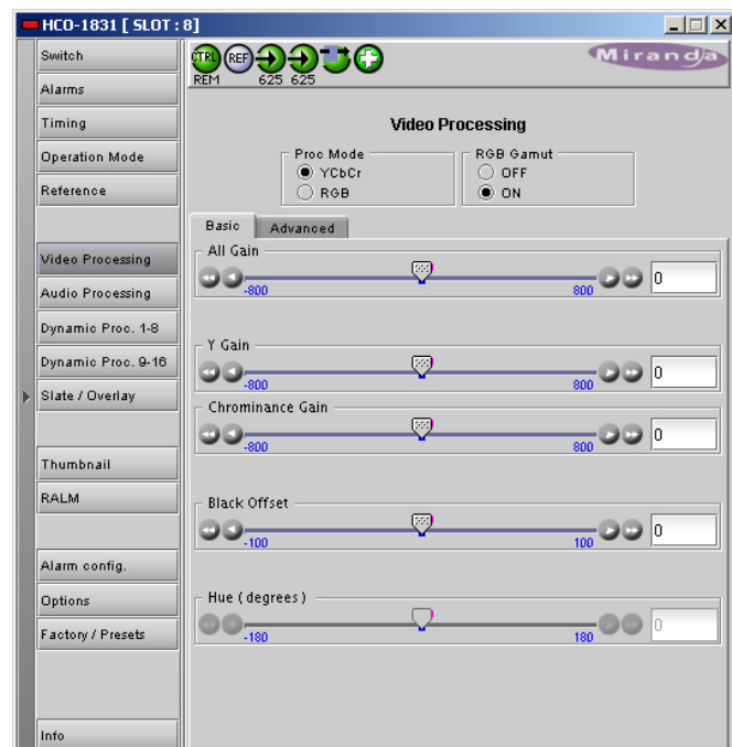
Figure 3.22 Video Processing panel – basic tab
