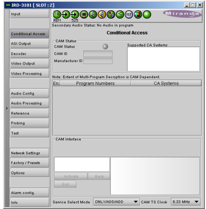
Figure 3.6 Conditional Access panel
