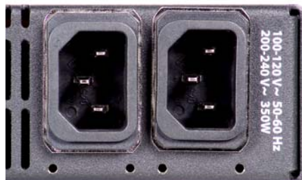
Fig. 12-12: Rear Panel Connectors - IEC Mains AC Inlets
