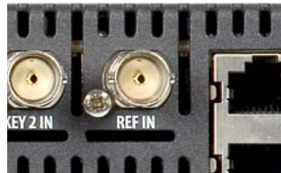
Fig. 12-3: Rear Panel Connector - REF Input
