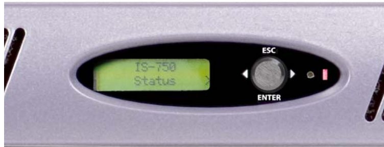
Fig. 12-13: Imagestore 750 Front Panel message after booting
