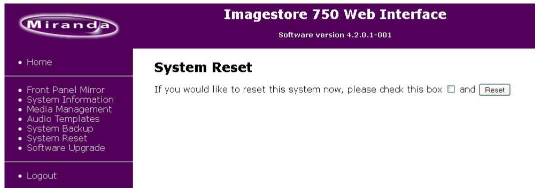
Fig. 9-9: Imagestore 750 Web Interface - System Reset
