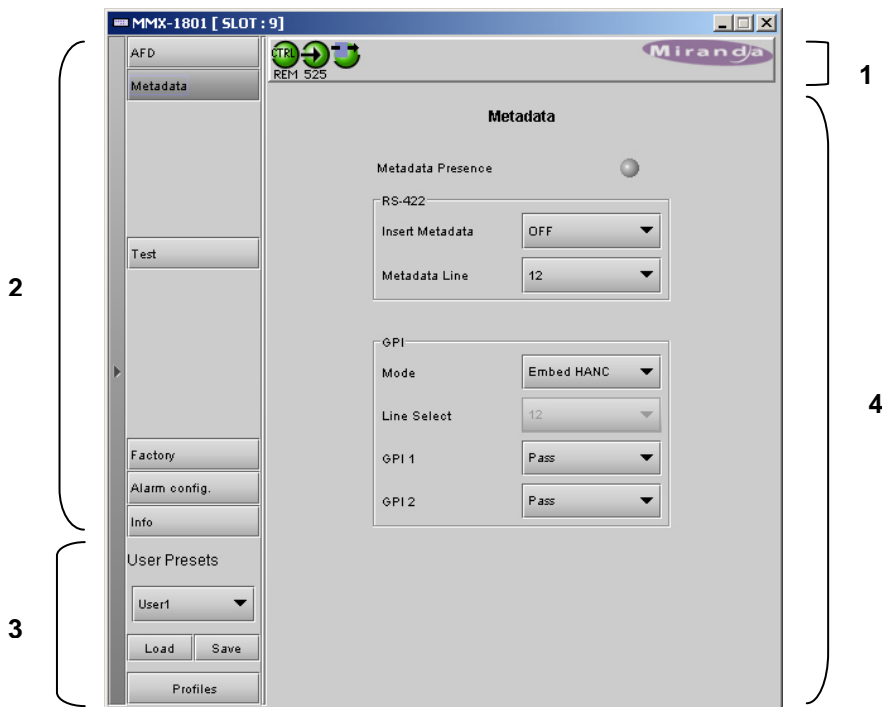
Figure 3.2 MMX-1801 iControl graphic interface window:
