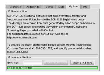
The Options tab explains the functionality of the IP scope option, and provides a data entry box "Enter Key" where
