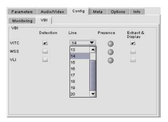
The SCP-1121 can detect and process three VBI data components:
