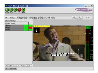
The display on the right side shows the thumbnail associated with the SDI video stream that is being monitored by the SCP-1121, and the audio level meter monitoring the audio in the data stream..
