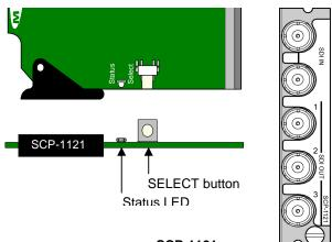
SCP-1121 Front card edge and Rear Connector Panel
