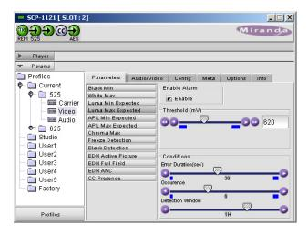
**On the left**, there is a tree chart of the eight Profiles available on the probe. A **Profile** is a set of values for all adjustable parameters and settings for the probe.
