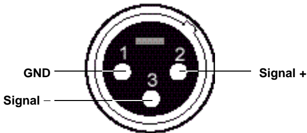
Figure 3.3 Male XLR connector pinout
