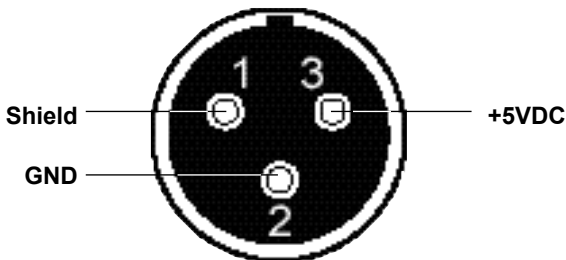
Figure 3 Power connector pinout
