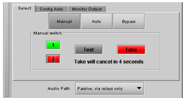
Figure 3.4 The Manual Switch Controls
