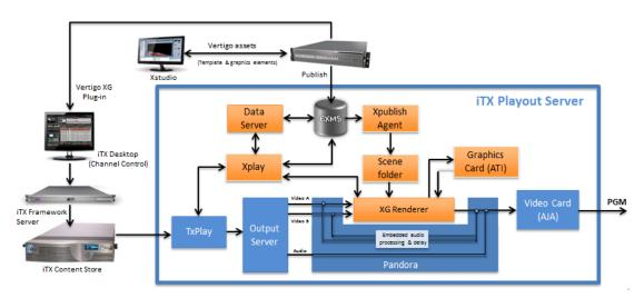
Figure 1-1. XG Inside signal path and workflow
