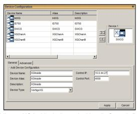
Figure 2-3. Adding an XG Inside device to the Xmedia Server's Device Manager
