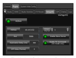
Figure 2-5. The VertigoXG plugin's configuration settings
