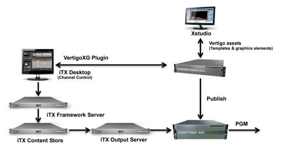
Figure 1-3. System diagram of an external Vertigo XG device downstream of an iTX system
