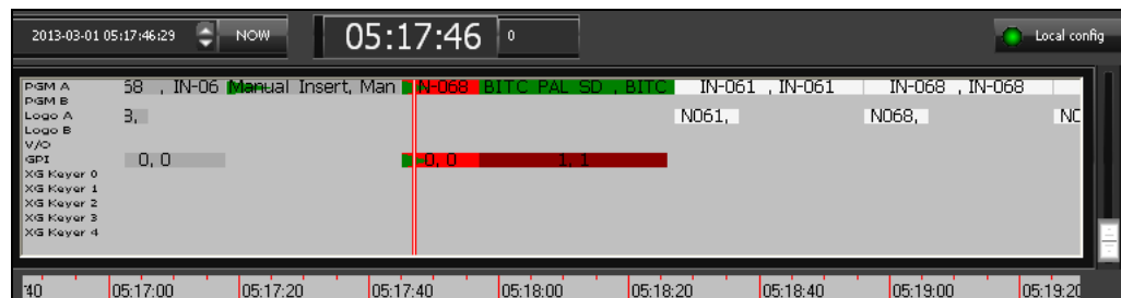
Fig. 5-1: A "Manual Insert" breaks into regular programming and resumes from the point of interruption
