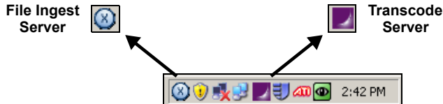
Figure 20-3. Once started the File Ingest Server icon appears in the notification area
