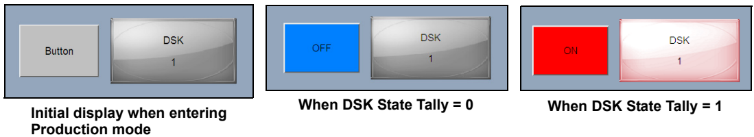
Figure 5-4. The button's expected behavior in Production mode when a DSK State tally is received
