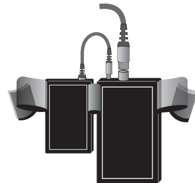
Auxiliary Battery Pack plugged into Power Pack and mounted on Tracking Ring Power Pack Belt
