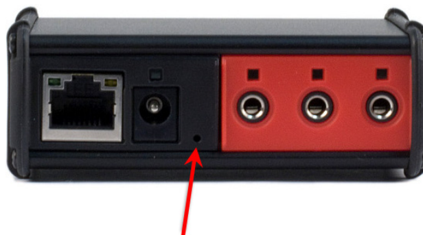
Figure 4-7: IR sensor (red arrow) on Global Caché iTach IP to IR device
