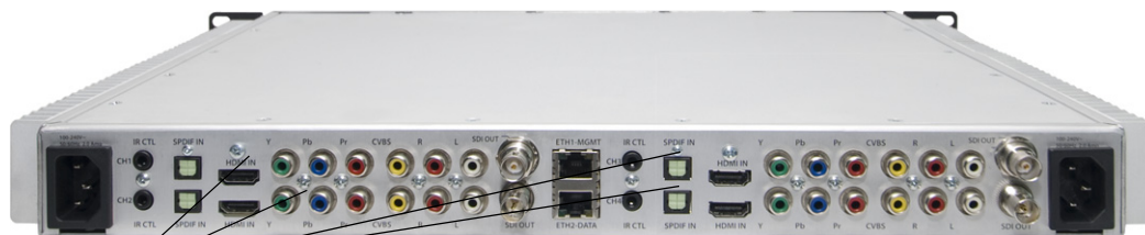
The EdgeVision device can have up to four sets of connectors, one for each input feed.
