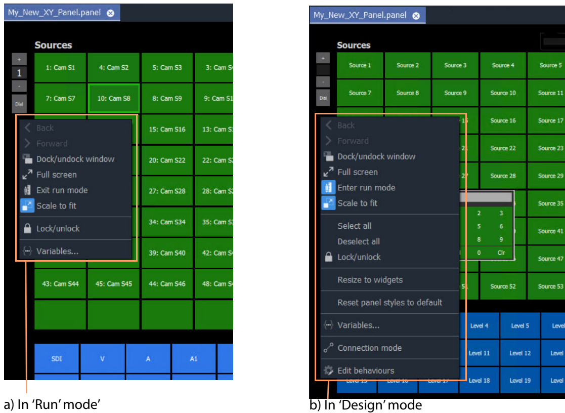
Fig. 3-14: XY Panel Background Right-Click Menu: a) in 'Run' Mode; b) in 'Design' Mode.
