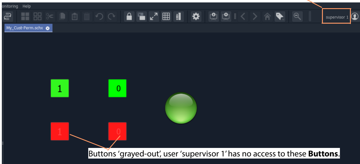
Fig. 4-26: C&M Screen Widget Access Control Example - Running: a) Logged in as 'administrator' role; b) logged in as 'supervisor' role.
