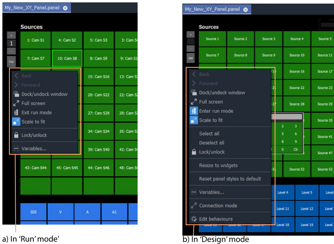
Fig. 6-16: XY Panel Background Right-Click Menu: a) in 'Run' Mode; b) in 'Design' Mode.
