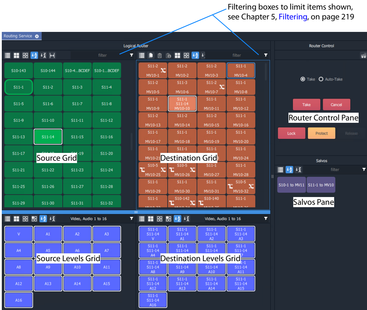
Fig. 3-28: Example Bulk Routing Panel
