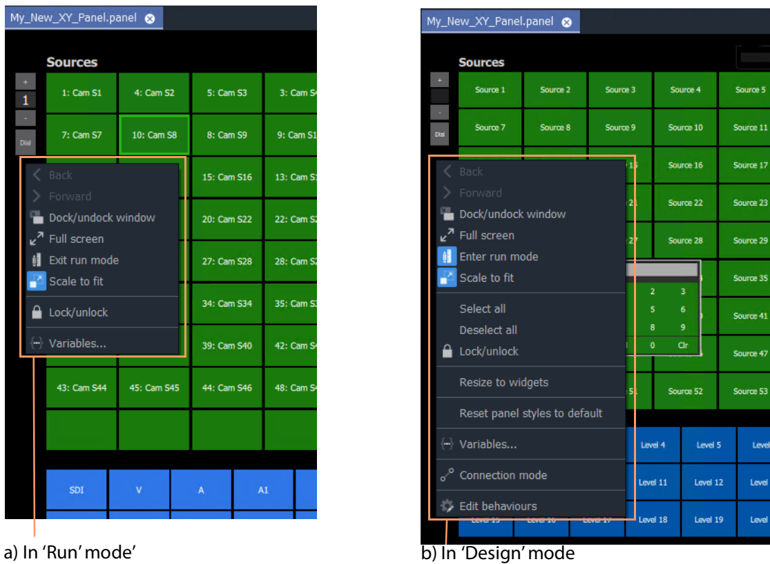
Fig. 12-16: XY Panel Background Right-Click Menu: a) in 'Run' Mode; b) in 'Design' Mode.
