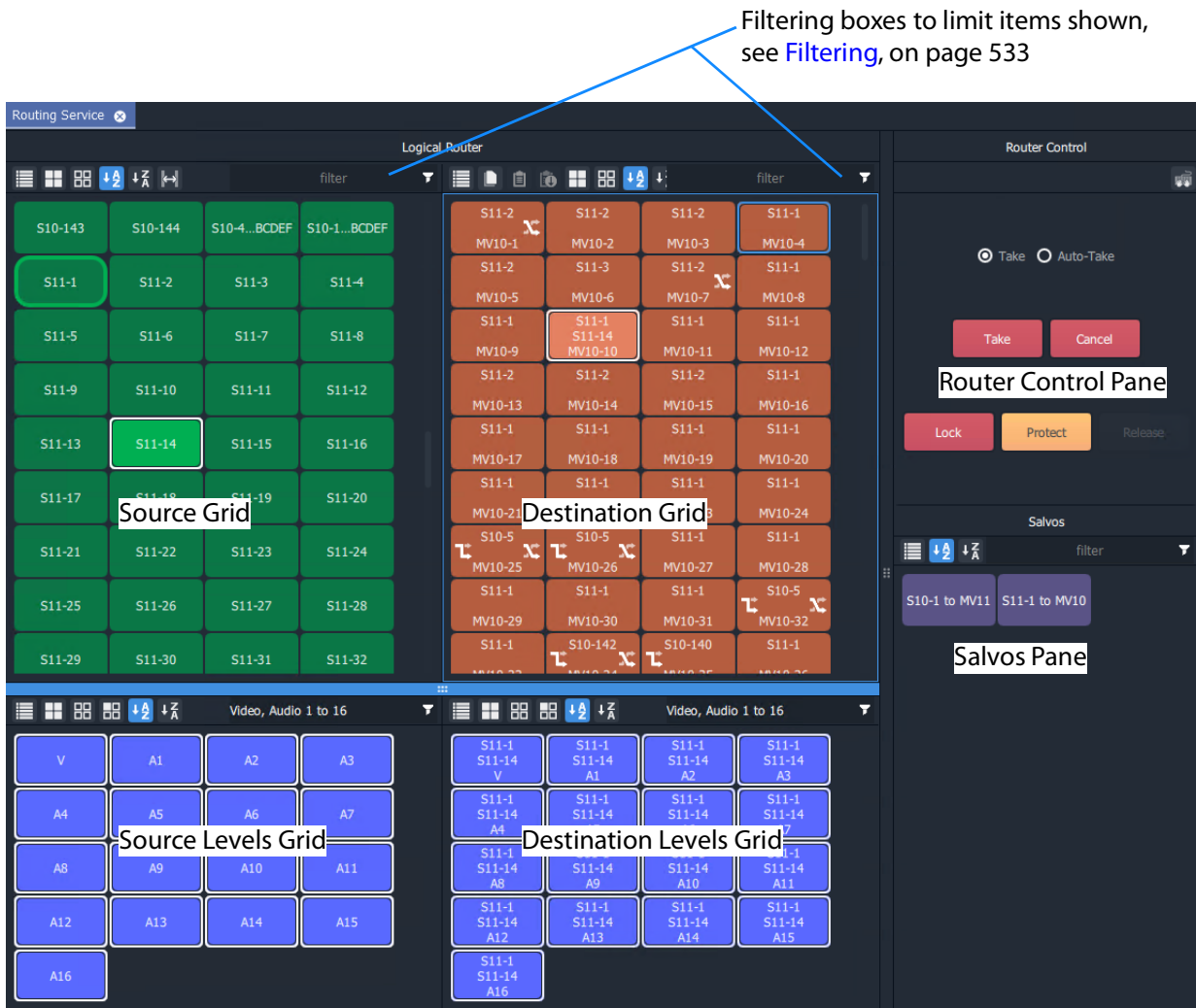
Fig. 3-28: Example Bulk Routing Panel
