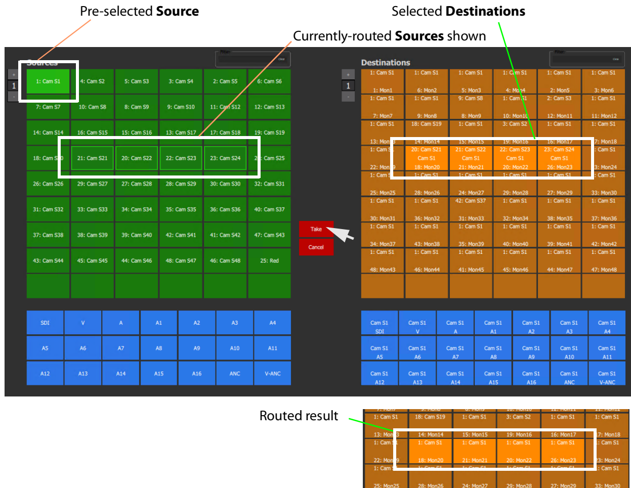
Fig. 12-22: One Source Routed to Multiple Destinations
