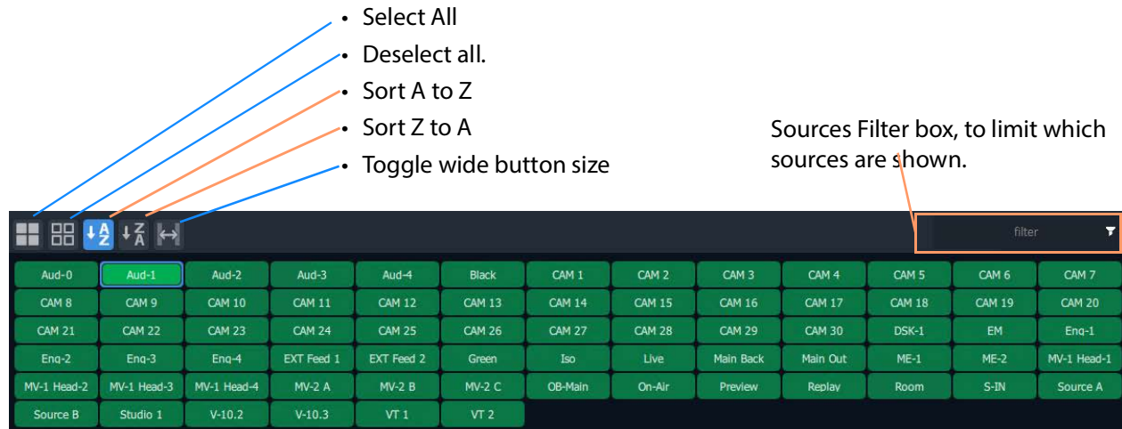
Fig. 15-82: Router Sources Grid Banner Tool Bar Controls
