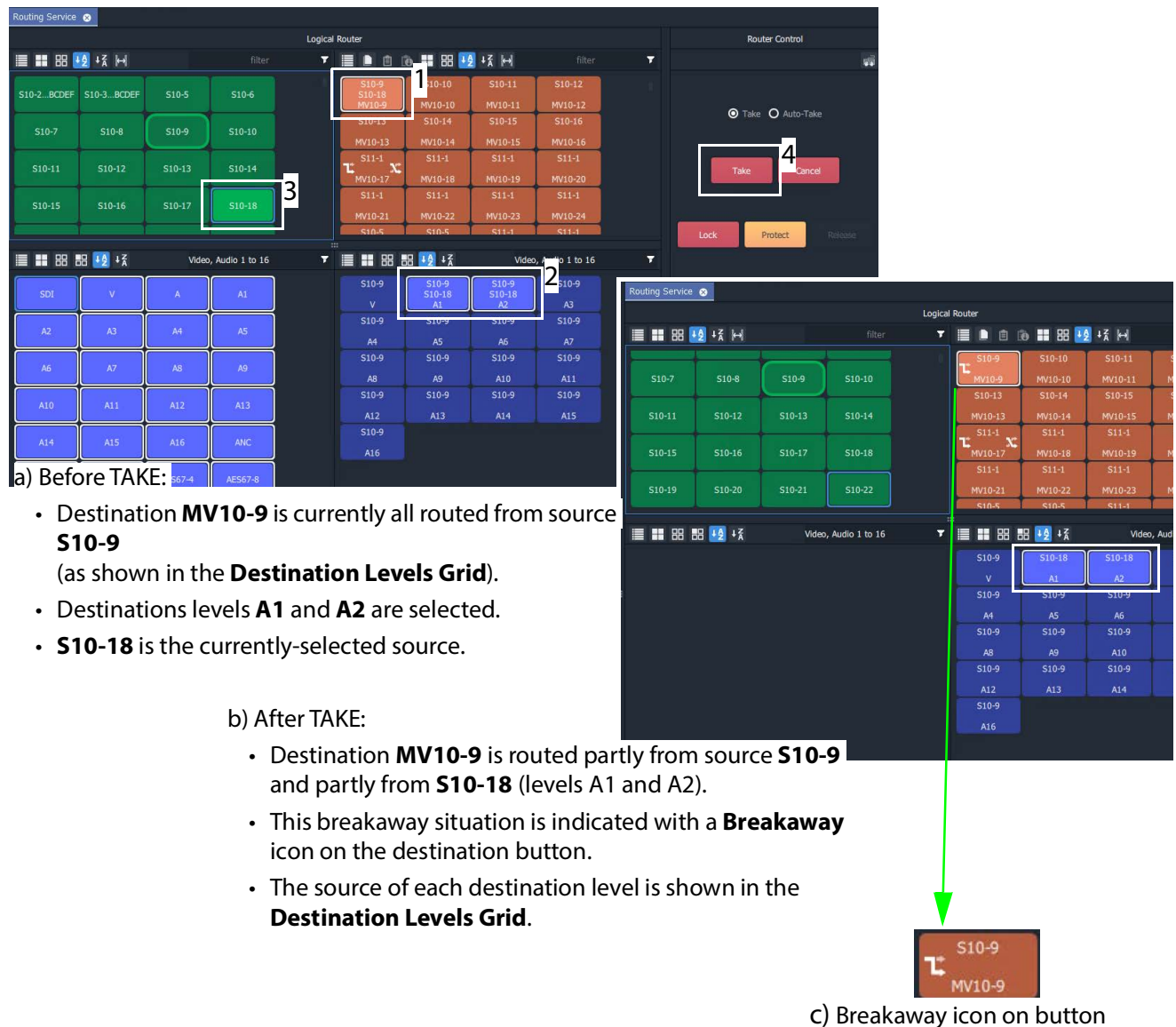
Fig. 12-33: Breakaway Example: a) Before TAKE; b) After TAKE; c) Breakaway Icon on Button.
