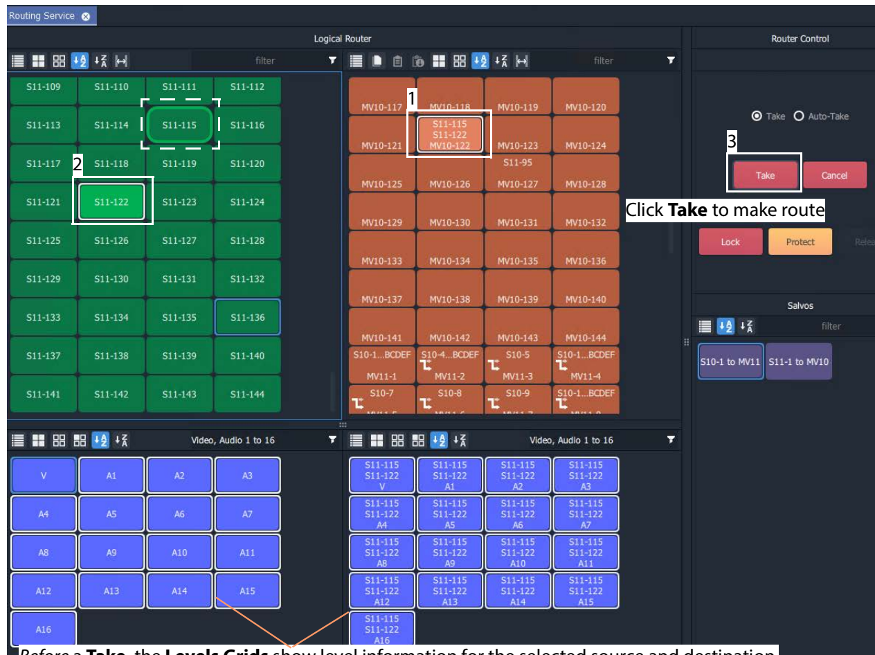
Before a Take , the Levels Grids show level information for the selected source and destination.
