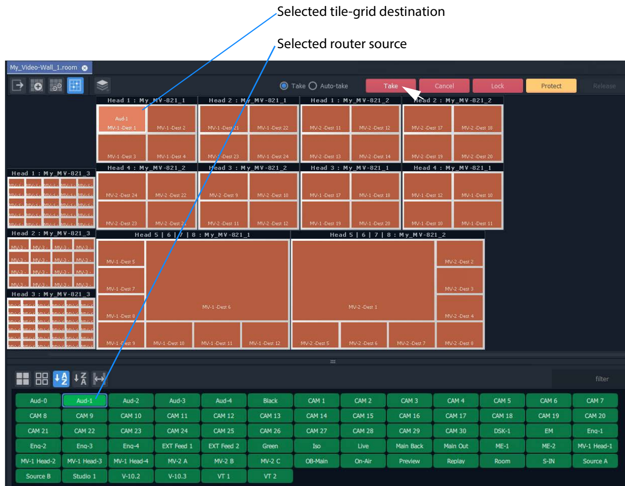
Fig. 15-83: Ready to Make a Router
