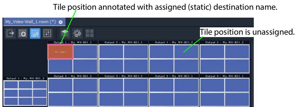
Fig. 15-69: Static Destination Assigned to Tile Position
