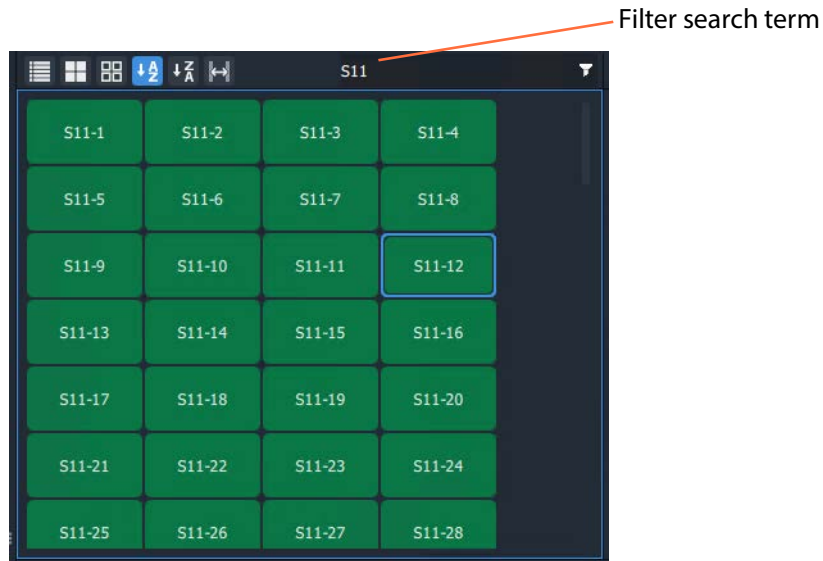
Fig. 12-44: Example of Simple Filtering Applied to a Grid/Pane (Search Term = "S11")
