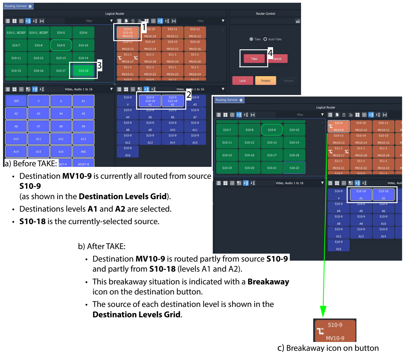
Fig. 13-33: Breakaway Example: a) Before TAKE; b) After TAKE; c) Breakaway Icon on Button.
