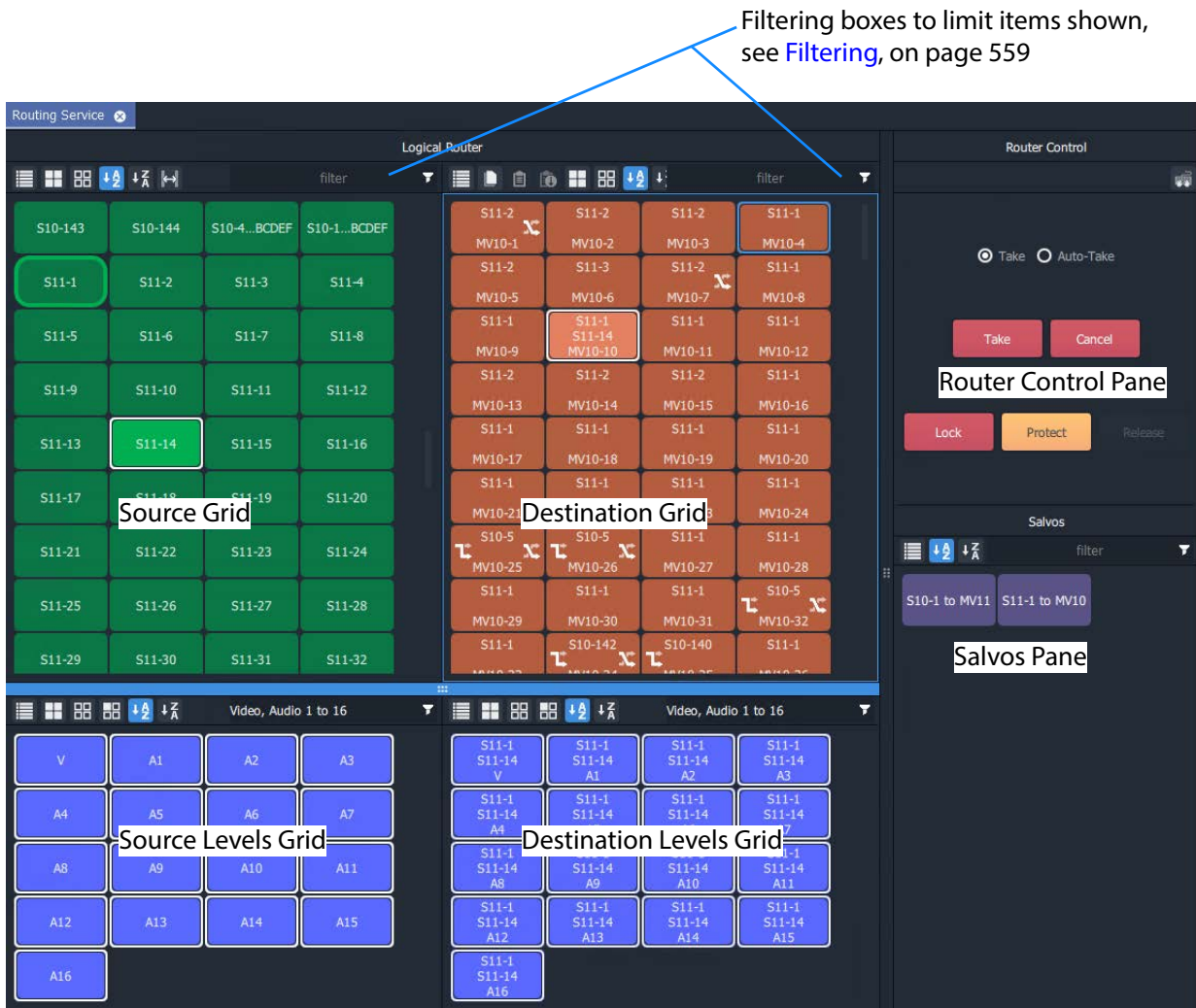
Fig. 3-21: Example Bulk Routing Panel
