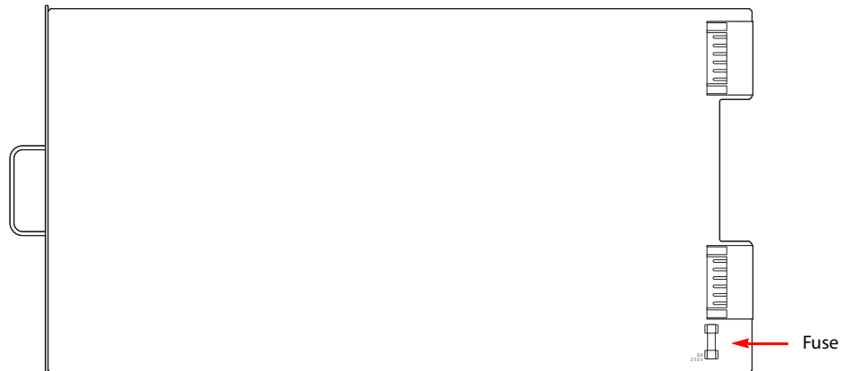
Figure 5-2. Fuse Location, PS6000 or PS6100 Power Supply
