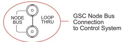
Figure 1-10. GSC Node Bus Connections to Router Control System (Rear View)
