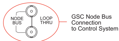
Figure 2-21. GSC Node Bus Connection to Control System (Rear View)
