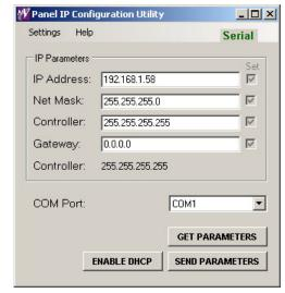
Both the IP address and the net mask are currently 0.0.0.0, indicating that the control panel is attempting to resolve its IP address through the use of a DHCP server. You must change both of these values to configure a static IP address. In this example, we used 192.168.1.58, and 255.255.255.0.
