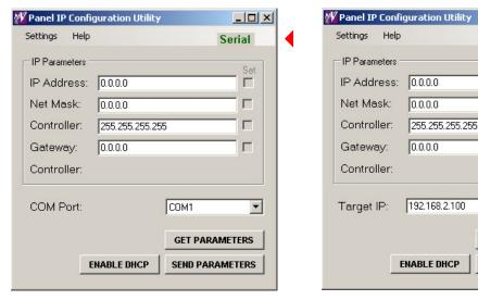
In serial mode, you can select the COM port through which the software will communicate with the control panel. Serial mode requires a direct connection between your PC and the control panel.
