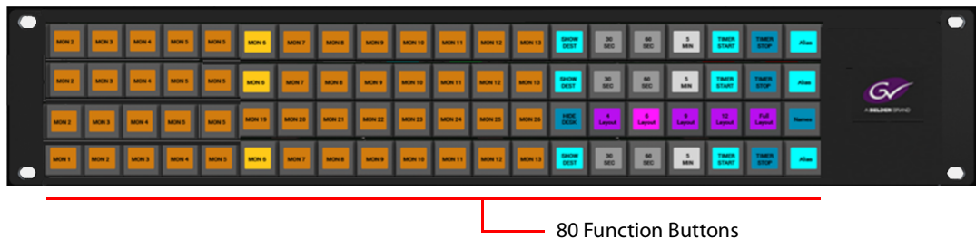
Fig. 2-1: NV9680 Front View
