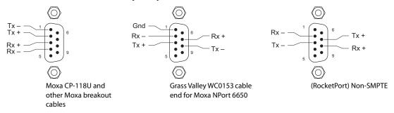
Your cabling must accommodate the pinout. In all cases, Tx- connects to Rx- and Tx+ to Rx+.
