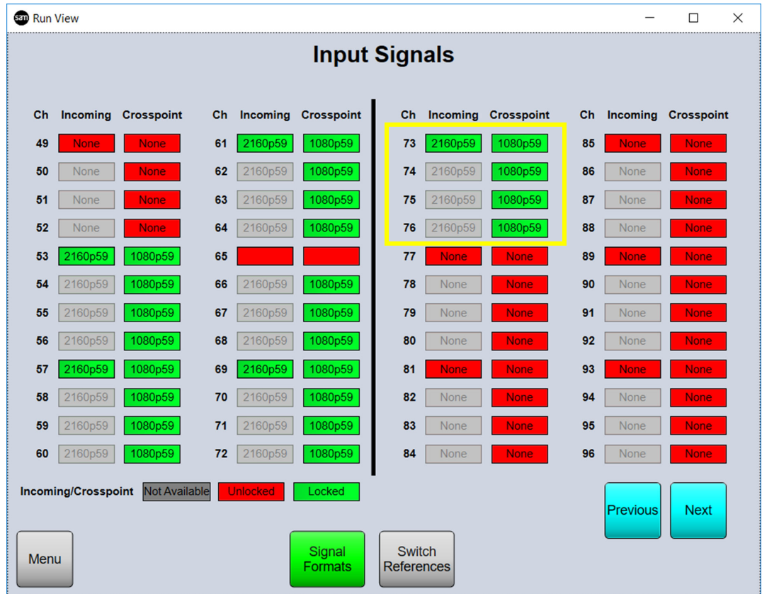
Figure 266 Router Input Signals Status Screen
