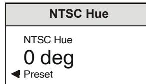
By using the spinwheel the Hue may be adjusted by ± 45 deg. in steps of 1degree.
