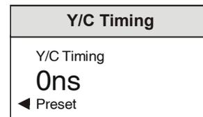
By using the spinwheel the timing may be adjusted by ± 592 ns in 148 ns steps.
