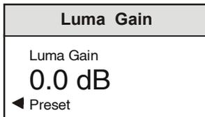
By using the spinwheel the gain may be adjusted by ± 6 dB in steps of 0.1 dB.
