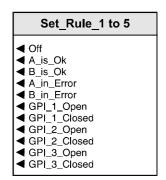
The Rule is set here to any one of 10 possibilities including input checking and GPI condition. 'Off' disables the Rule.
