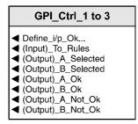
This menu should be used to select the operation of each GPI port. If a GPI input is used in any of the Rule definitions then it **must** be set to (Input)\_To\_Rules
