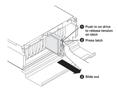
When installing a media drive, push it in firmly and make sure that it clicks into place completely.
