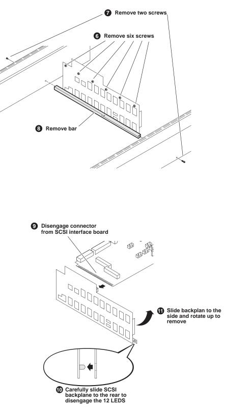
When installing replacement, ensure the LED solder ends clear the cut outs and are not shorting against the bracket.
