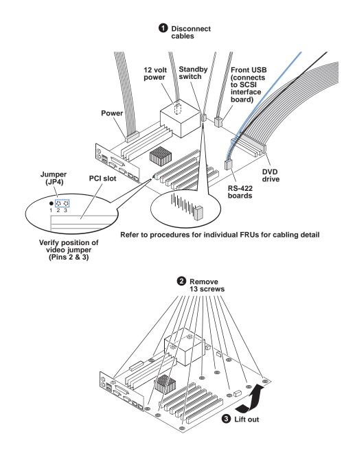
Save the connector panel to exchange with the replacement motherboard. When installing the replacement motherboard, first install the connector panel on the motherboard, being careful to engage flanges on connectors. Then install the motherboard in the chassis, making sure the connector panel "snaps" into the chassis on all edges.
