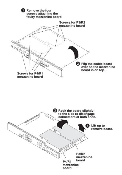
NOTE: Make sure the replacement board is the same type (encoder or decoder) and installs in the same position as the faulty board. Changing the type, position, or number of encoder/decoder mezzanine boards renders the K2 Media Client inoperable.
