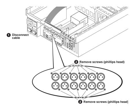
When installing the replacement XLR board, apply pressure as you insert the screws as the screws must cut their own threads.
