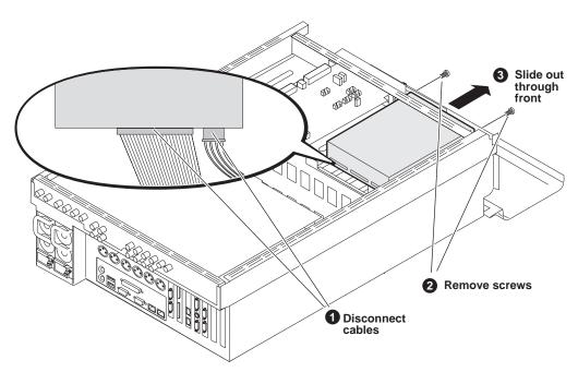
For the CD drive, you must exchange the brackets with the replacement unit, as in the following illustration.
