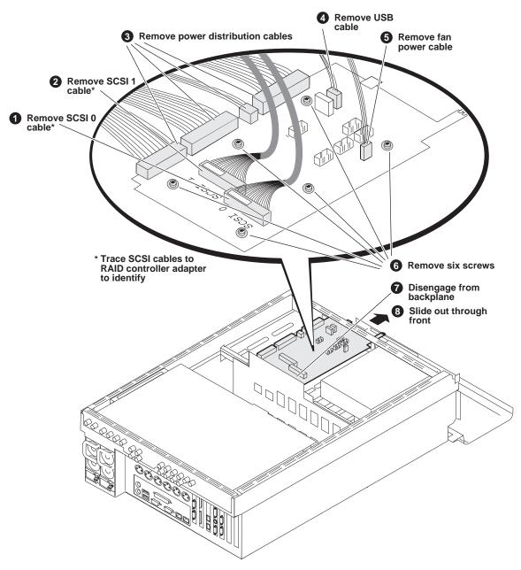
Refer to "SCSI controller adapter removal" on page 114 for cable detail on RAID controller adapter to identify SCSI 0 and SCSI 1 cables.
