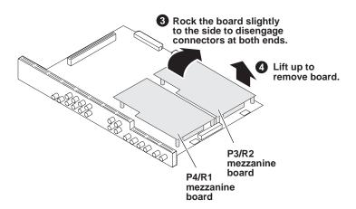
NOTE: Make sure the replacement board is the same type (encoder or decoder) and installs in the same position as the faulty board. Changing the type, position, or number of encoder/decoder mezzanine boards renders the K2 Media Client inoperable.
