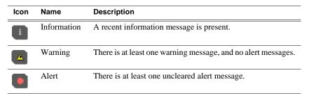
Current and previous system status messages can be viewed in the StatusPane. To open the StatusPane, click **Help | System Status**.
