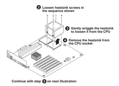
NOTE: On the Type II motherboard, the CPU is in slot 2.
