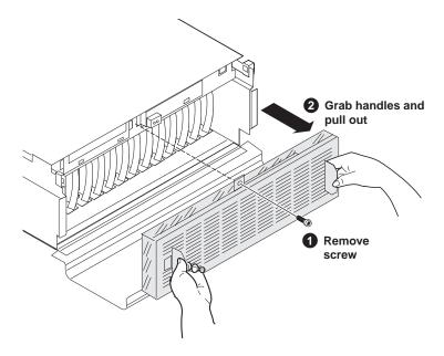
You can remove the fan module while the K2 Media Client is operating. If you do so, make sure you replace it within one minute to ensure that the correct operating temperature is maintained.
