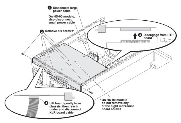
The codec board in HD-00 models is a different size than the codec board in the other models. On HD-00 models the codec board is wider, as shown. This requires that the RTP board be in rear slot two. On SD-00 models and on SDA-00 models, the codec board is narrower, which requires that the RTP board be in rear slot five. Take this into consideration when removing a codec board.
