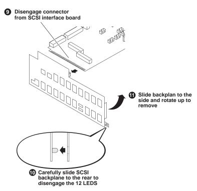
When installing replacement, ensure the LED solder ends clear the cut outs and are not shorting against the bracket.
