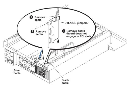
The RS-422 adapter in rear slot seven has the blue cable. The RS-422 adapter in rear slot three has the black cable. All models have RS-422 adapters in these rear panel slots (slot three and slot seven).
