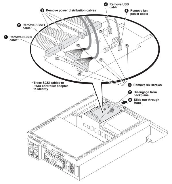
Refer to "SCSI controller adapter removal" on page 121 for cable detail on RAID controller adapter to identify SCSI 0 and SCSI 1 cables.
