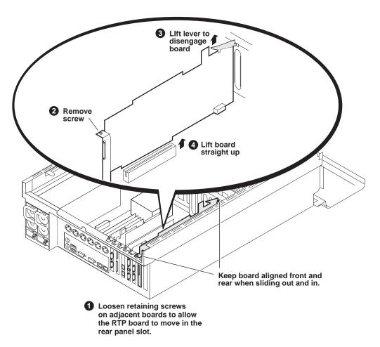
On HD-00 models the RTP board is in rear panel slot two, as shown. On other models the RTP board is in rear panel slot five.
