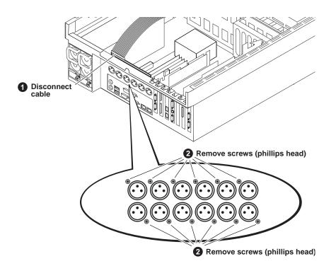
When installing the replacement XLR board, apply pressure as you insert the screws as the screws must cut their own threads.
