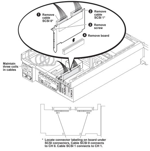
On all models the RAID controller adapter is in rear panel slot six, as shown.
