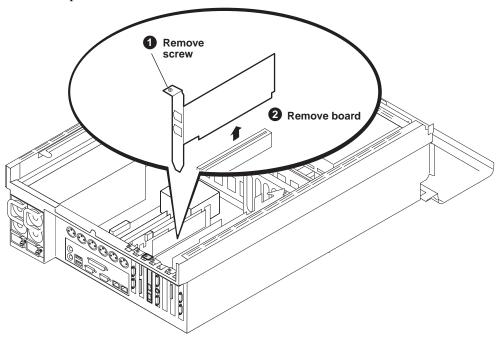
On HD-00 models the Dual Ethernet adapter is in rear panel slot five, as shown. On other models the Dual Ethernet adapter is in rear panel slot two.
