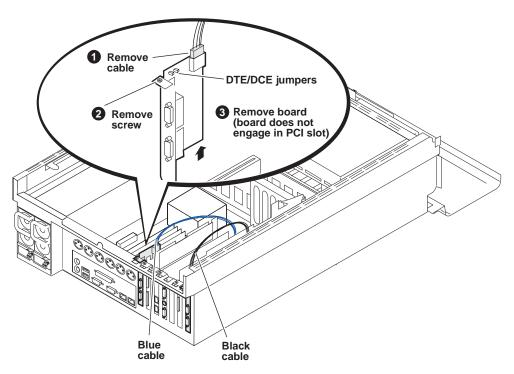
The RS-422 adapter in rear slot seven has the blue cable. The RS-422 adapter in rear slot one or three has the black cable. Refer to "Remove faulty motherboard" on page 127 for detail of USB connections to motherboard.
