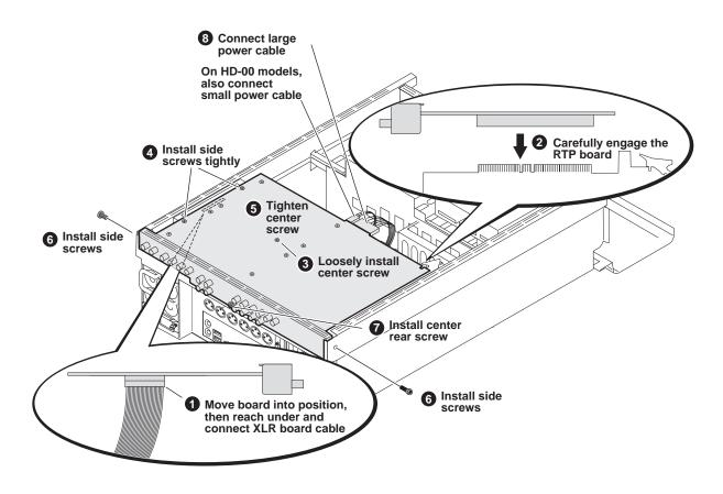
When installing the replacement board, make sure screws are installed in the proper sequence, as illustrated:
