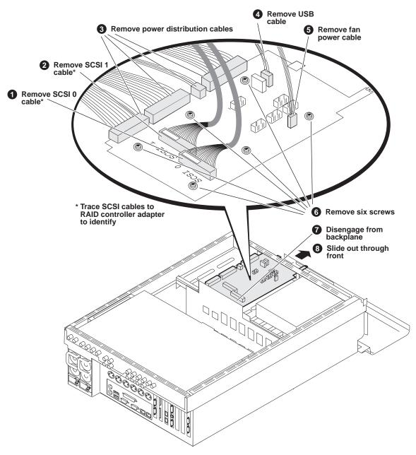
Refer to "SCSI controller adapter removal" on page 121 for cable detail on RAID controller adapter to identify SCSI 0 and SCSI 1 cables.
