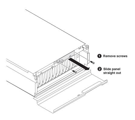
You must remove the front panel before removing the SCSI interface board.
