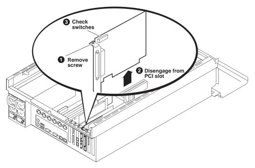
On the replacement RS-422 adapter, verify that the switches that set channels to Data Terminal Emulation (DTE) or Data Communications Emulation (DCE) are in the same position as those on the adapter that you are replacing.
