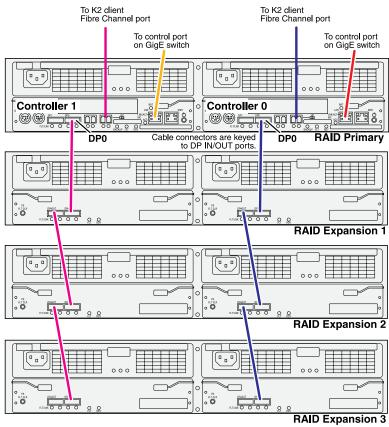
NOTE: Do not connect the controller MNT port. It should only be used with a PC in a peer-to-peer connection for diagnostics purposes.
