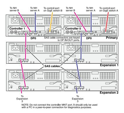
For the Nearline system, if you have more Expansion chassis than those illustrated, continue the indicated cabling pattern, alternating connections for additional Expansion chassis between DP1 and DP0. Expansion chassis 1, 3, 5, etc. connect to DP1. Expansion chassis 2, 4, 6, etc. connect to DP0.
